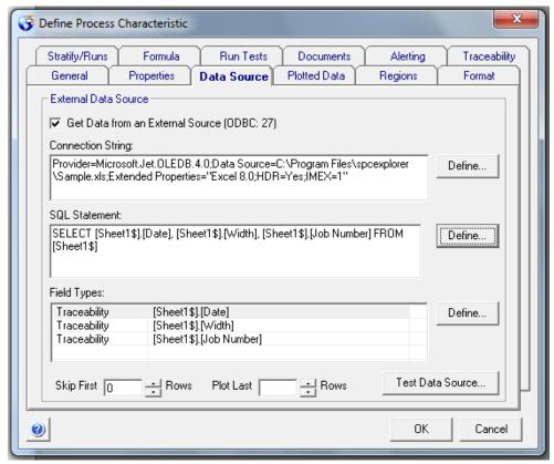
9. Here, you will set up the various fields you've selected to link. These fields will be set to Date fields, Data values, Traceability fields, etc. Highlight the field on the left and then select its appropriate type on the right (using the buttons). Click "OK" once you've assigned the different types to all the fields.
